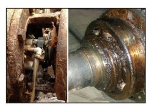
Bearing failed frequently in slurry pumps.
